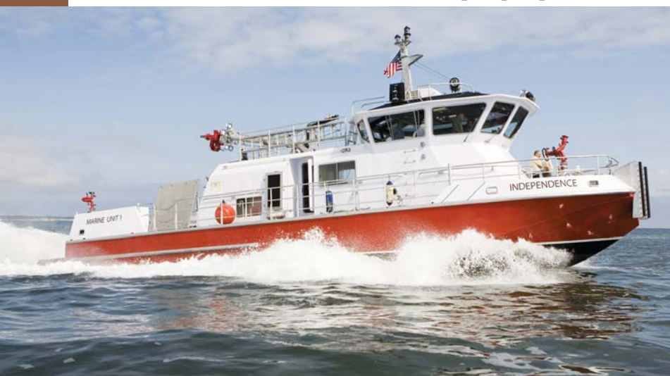
The Independence, a fire and rescue boat, has a navigation mast mounted to the top of its pilot house that pivots downward when the vessel must pass under a low clearance. The mast is pivoted 180° by a helical rotary actuator.
